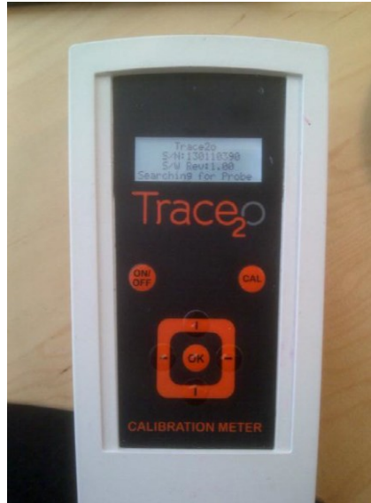
Figure 10 The calibration device, used for calibration of the probe
